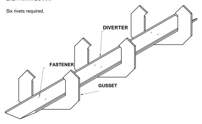
If the vent includes a damper, set up the damper guide rod into the damper guides with push-nut fasteners at the end of the rod. Attach the damper guide assembly to the diverter using two 3/16 X 1/4 rivets with closed ends.
