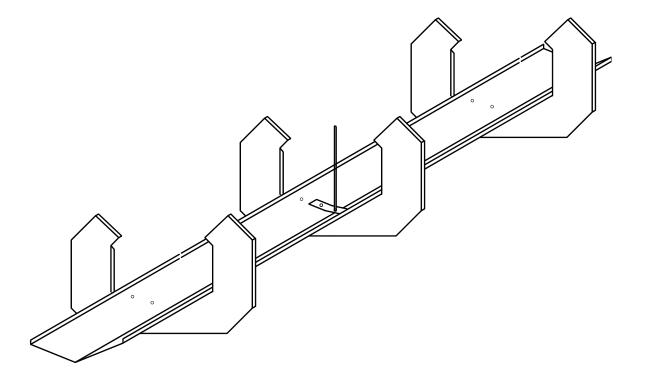
Set up the damper with one Heyco guide rod bushing, and the one damper horizontal guide assembly. Use two 3/16 X 1/4 rivets PART#AB64A.
