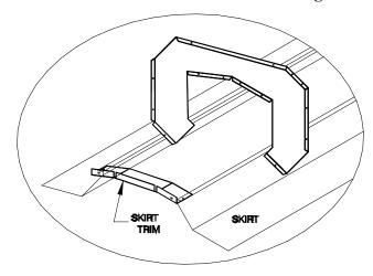
Attach the End Caps to the end of the vents with the windbands overlapping the flanges on the endcaps. Fasten using 3/16" rivets. Attach skirt and diverter trims to the end caps with 3/16" rivets.
