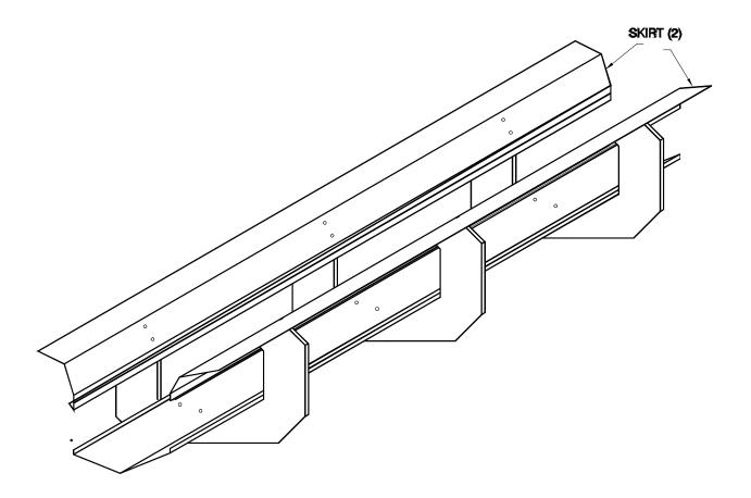
Position the braces over the top of the skirts in the orientation shown (windbands and end caps omitted for clarity). The middle brace is unique with a pathway and keeper provided for the chain operator and guide rod. Using 3/16 closed end rivets, fasten the skirts and braces to the gussets. 12 Rivets are required.
