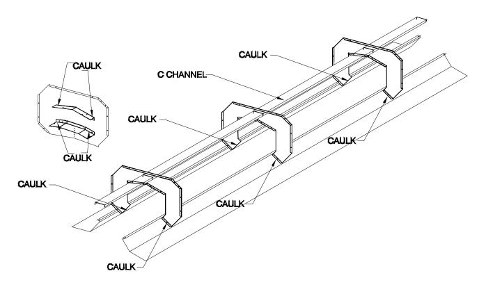
Turn the vent over 180 degrees. Attach the C Channel lifting arm. Fasten to each gusset. Caulk the End Cap to the Diverter Trim using the polyurethane caulking.
