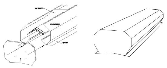
Caulk the Skirt Trim and skirt/end cap joints using the polyurethane caulking.
