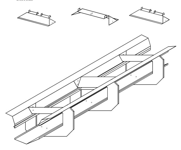
While in the up side down position, form the Diverter Trim by hand to match the shape of the water diverter and fasten one to each end of the diverter using 3/16" rivets. (Drawings shown in right side up position.)
