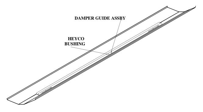
Place damper assembly over guide rods and diverter.
