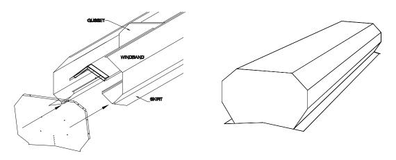
RV9 and RV12 Models – Caulk the Skirt Trim using the polyurethane caulking.
