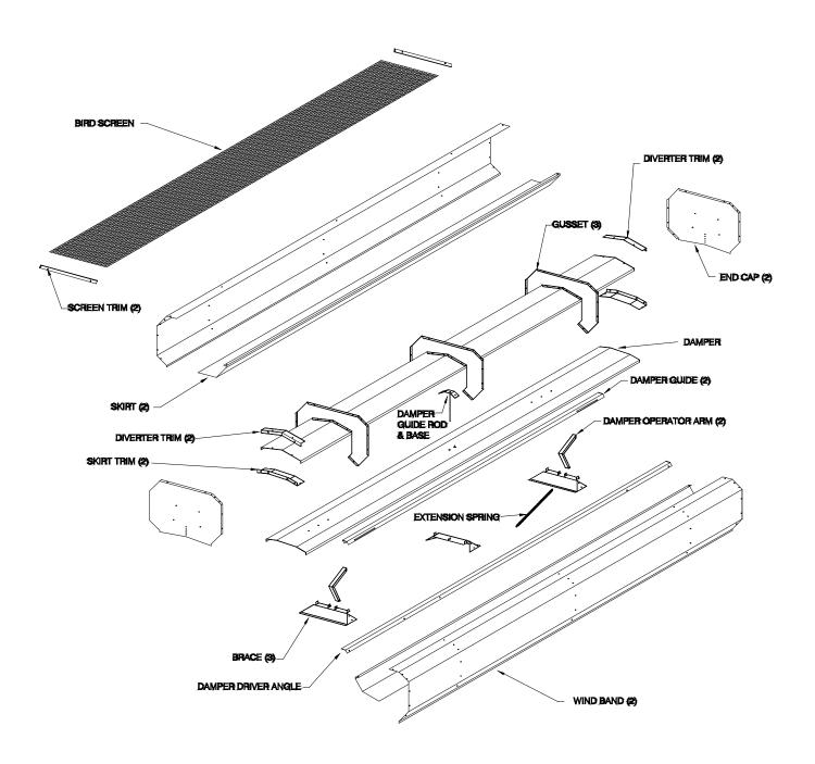
Lay the three gussets on a table with all 3 pieces facing the same direction spaced about 3 feet apart. Lay the diverter on top of the gussets. Tip the gussets up one at a time with the "horseshoe" facing up and fasten the diverter to the gussets with 1/8 X 1/8 ALUMINUM/ STEEL POP RIVET WITH CLOSED END PART#AB42CLD (RV-9 only). For the RV-12 and up, use 3/16 X 1/4 ALL ALUMINUM POP RIVET WITH CLOSED END PART#AD64AH. Six rivets required.
