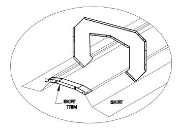
Attach the End Caps to the end of the vents with the windbands overlapping the flanges on the endcaps. Fasten using 1/8" rivets. Attach skirt and dievrter trims to the end caps.
