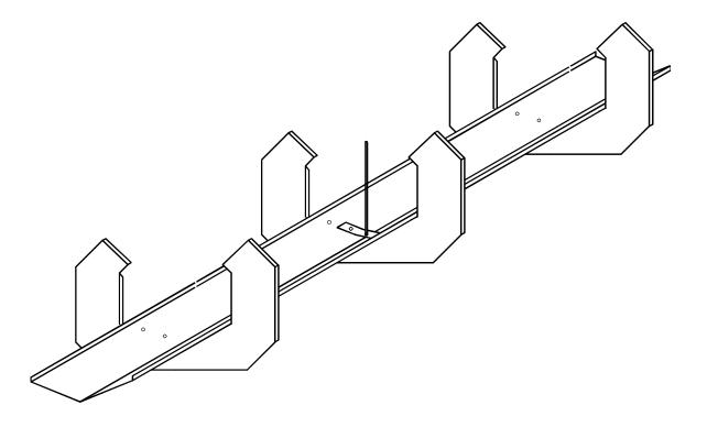
Set up the damper with one Heyco guide rod bushing, and the one damper horizontal guide assembly. Use two  $3/16~\rm X~1/4$  rivets PART#AB64A.
