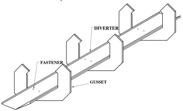
If the vent includes a damper, set up the damper guide rod into the damper guides with pushnut fasteners at the end of the rod. Attach the damper guide assembly to the diverter using two  $3/16 \times 1/4$  Rivet with closed ends.
